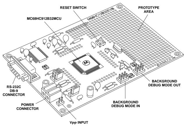
**Figure 1. Evaluation Board Layout**
